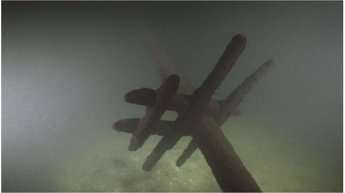
Fig. 8. Mizzen topmast crosstrees. Frame capture from video by Immi Wallin.
