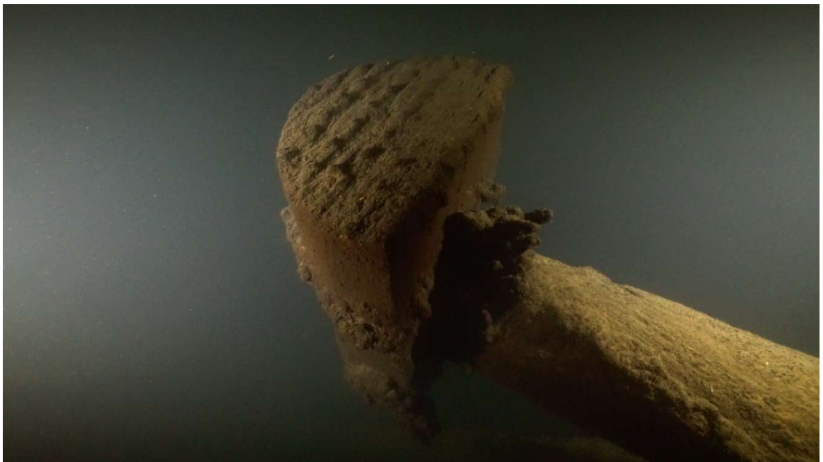
Fig. 7. Mizzen mastcap. Frame capture from video by Immi Wallin.
