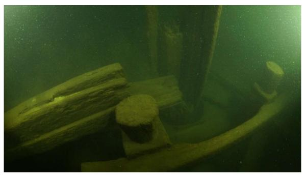
Fig. 39. Jeerbitts behind the main mast. Video frame capture: Kari Hyttinen.
