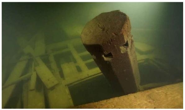
Fig. 38. The upper part of the capstan behind the foremast with 8 holes. Video frame capture: Kari Hyttinen.
